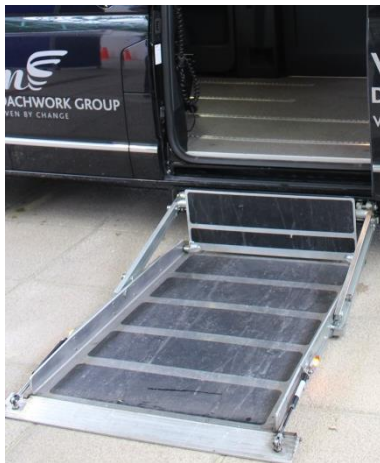
Figure 26: Non perforated lift platform material
