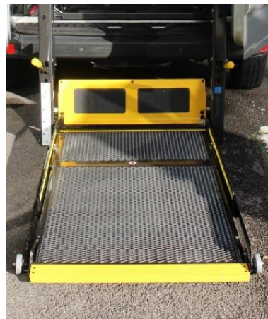
Figure 27: Perforated lattice like lift platform material
